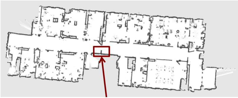
Figure 4.4: A grid map (also called an occupancy grid) is a large gray-scale image, each pixel represents a cell in the physical world. In this picture, cells that are occupied are colored black and empty cells represent free space. A grid map is a useful representation for a robot to localize in this house using observations from its sensors and comparing those to the map.
