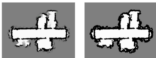
Figure 4.6: (Left) A typical occupancy grid created using a sonar sensor by updating the log-odds-ratio l(m_i | x_{1:k}, y_{1:k}) for all cells i for multiple time-steps k . At the end of the map building process, if l(m_i | x_{1:k}, y_{1:k}) > 0 for a particular cell, we set its occupancy to 1 and to zero otherwise, to get the maximum-likelihood estimate of the occupancy grid on the right.
