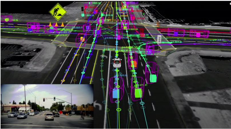
Figure 4.7: The output of perception modules for a typical autonomous vehicle (taken from https://www.youtube.com/watch?v=tiwVMrTLUWg ). The global occupancy grid is shown in gray (see the sides of the road). The local map is not shown in this picture but you can imagine that it has occupied voxels at all places where there are vehicles (purple boxes) and other stationary objects such as traffic light, nearby buildings etc. Typically, if we know that so and so voxel corresponds to a vehicle, we run an Extended Kalman Filter for that particular vehicle to estimate the voxels in the local map that it is likely to be in, in the next time-instant. The local map is a highly dynamic data structure that is rich in information necessary for planning trajectories of the robot.
